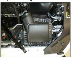
6. Pull the factory air filter housing straight up and remove it from the vehicle. **NOTE: K&N Engineering, Inc., recommends that customers do not discard factory air intake.**
