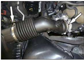
4. Loosen the hose clamps that secure the factory intake tube and then remove the intake tube from the vehicle.
