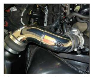
16. Install the intake tube into the couplers, position for best fit and then secure with the provided hose clamps.
