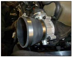
13. Install the step coupler onto the throttle body and secure with the provided hardware.
