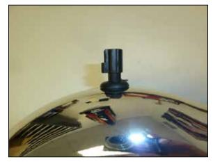
15. Remove the IAT sensor from the factory intake tube and then remove the O-Ring from the sensor. Using the provided grommet, install the sensor into the K&N intake tube as shown. **NOTE: The IAT sensor is very fragile, use caution while handling the sensor so as not to damage it.**
