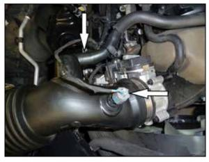
3. Disconnect the IAT sensor electrical connection and unhook the wiring harness from intake tube. Then disconnect the CCV hose from the intake tube.
